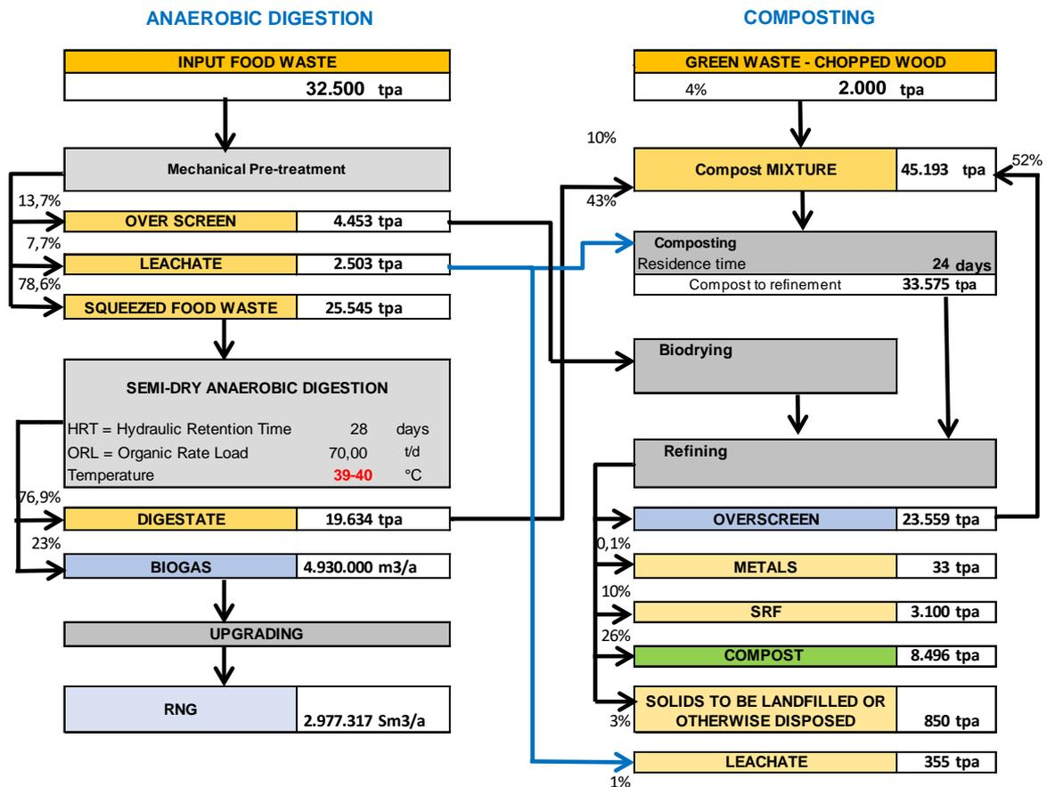
Fig. 4. Block diagram of plant mass balance
