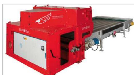
(2) **SEPARATORE NIR FALCON PER RIMUOVERE PLASTICHE CLORATE**
