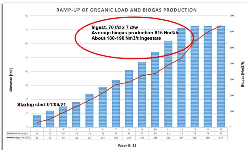
Fig. 2. Ramp up: feeding ratio vs. biogas production
