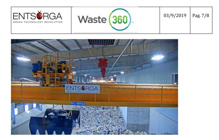
Entsorga makes an engineered fuel it calls Prometheus. Prometheus can be produced according to customer's specifications by biodrying municipal solid waste, mechanically refining it and possibly adding selected commercial and industrial waste. This is done to homogenize the chemical composition and raise British thermal unit content, says Paolo Carollo, vice president of operations for North America at Entsorga.
